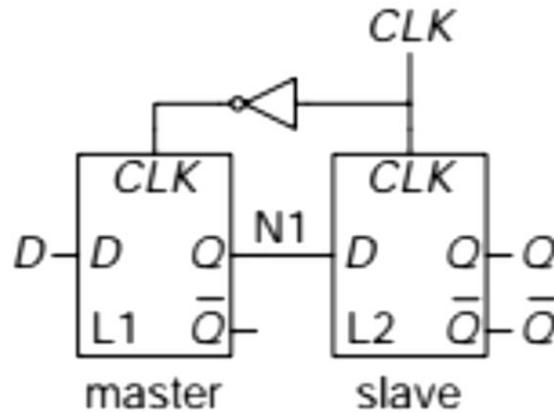
Figure 3: D-flip flop
